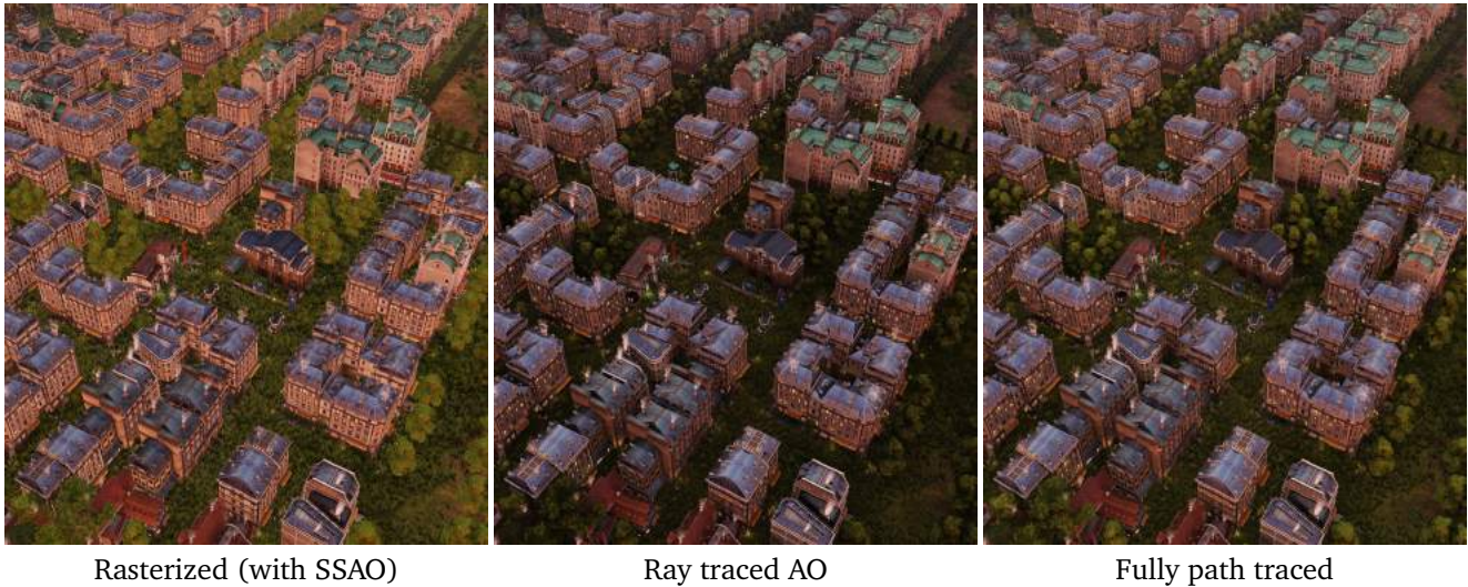
Figure 4.19: Comparison of an Anno city scene at sunset with different indirect lighting strategies.
