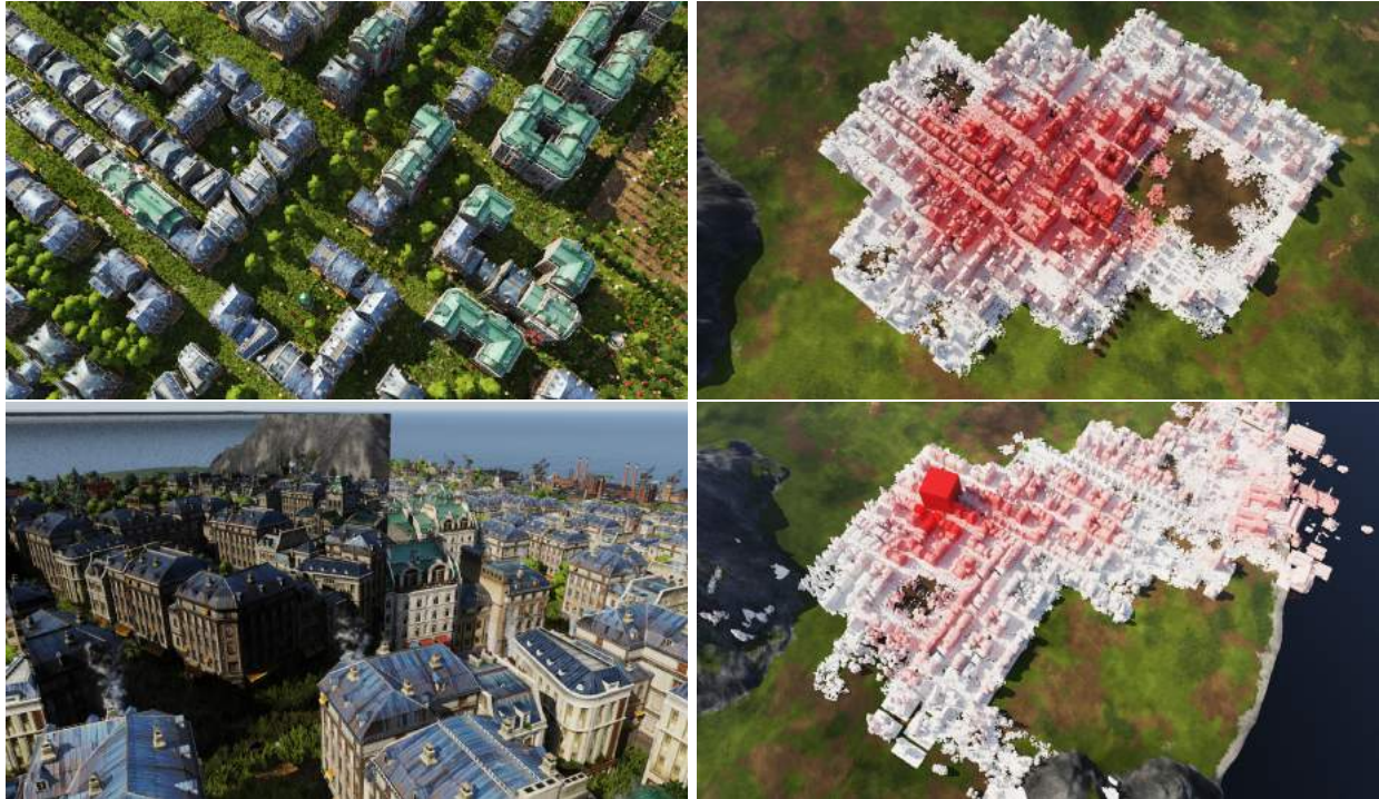
Figure 3.3: Visualized hit feedback in a big city scene. Left: path traced views of the scene. Right: the instances present in the TLAS for the associated perspective on the left. In the second row, a mirroring cube was placed into the scene. Object color is interpolated from white to red, the higher the hit count.
