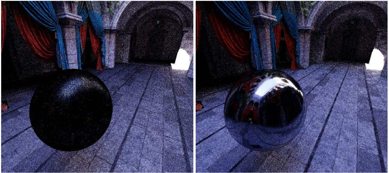
Figure 2.1: The importance of importance sampling. Sponza with a mirroring ball, 10 samples per pixel (spp). Left: No importance BRDF sampling applied, as outlined by algorithm 2 . Right: With BRDF importance sampling, as outlined by algorithm 3 .
