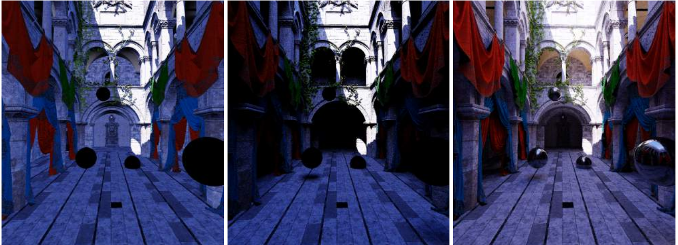
Figure 1.1: Differently shaded Sponza [Int22] scene with added reflective curved surfaces. Left: Approximating indirect diffuse lighting with a trivial position-independent term Middle: Ray traced ambient occlusion (AO), correctly computing light coming from the sky. Right: Fully path traced image showing accurate indirect lighting.
