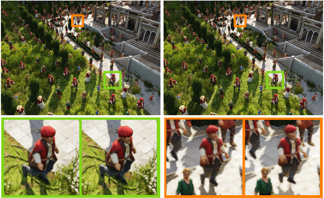
Fig. 9. Lighting and shadow comparison. Left: Ground Truth. Right: LiPaC with high activation thresholds, falling back on rasterized shadows for omitted models.
