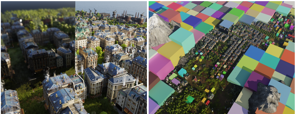
Fig. 3. Visualized hit feedback. Left: path traced views of the scene. Right: the instances present in the TLAS for the associated perspective on the left.
